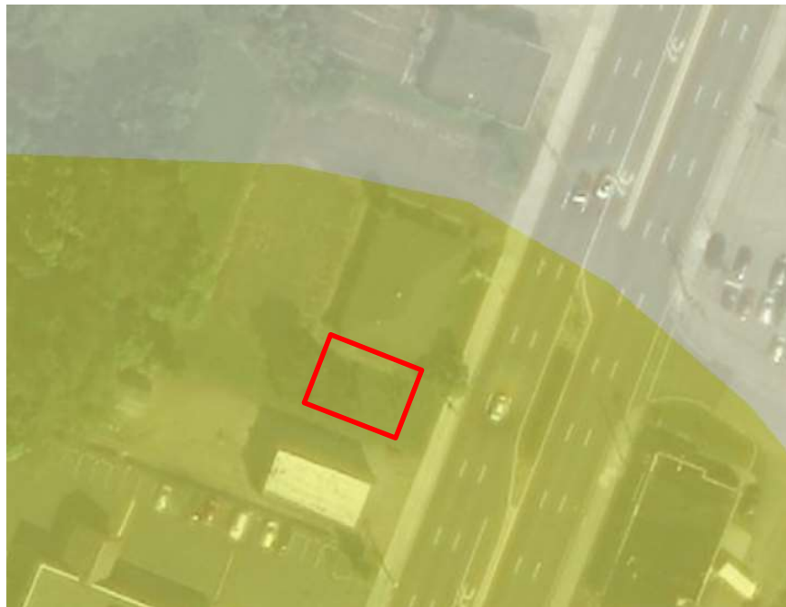
Figure 7: The site is located near the transition between glacial outwash deposits (yellow shading) and alluvium (white shading). However, the addition (red) is reportedly underlain by the outwash deposits.
