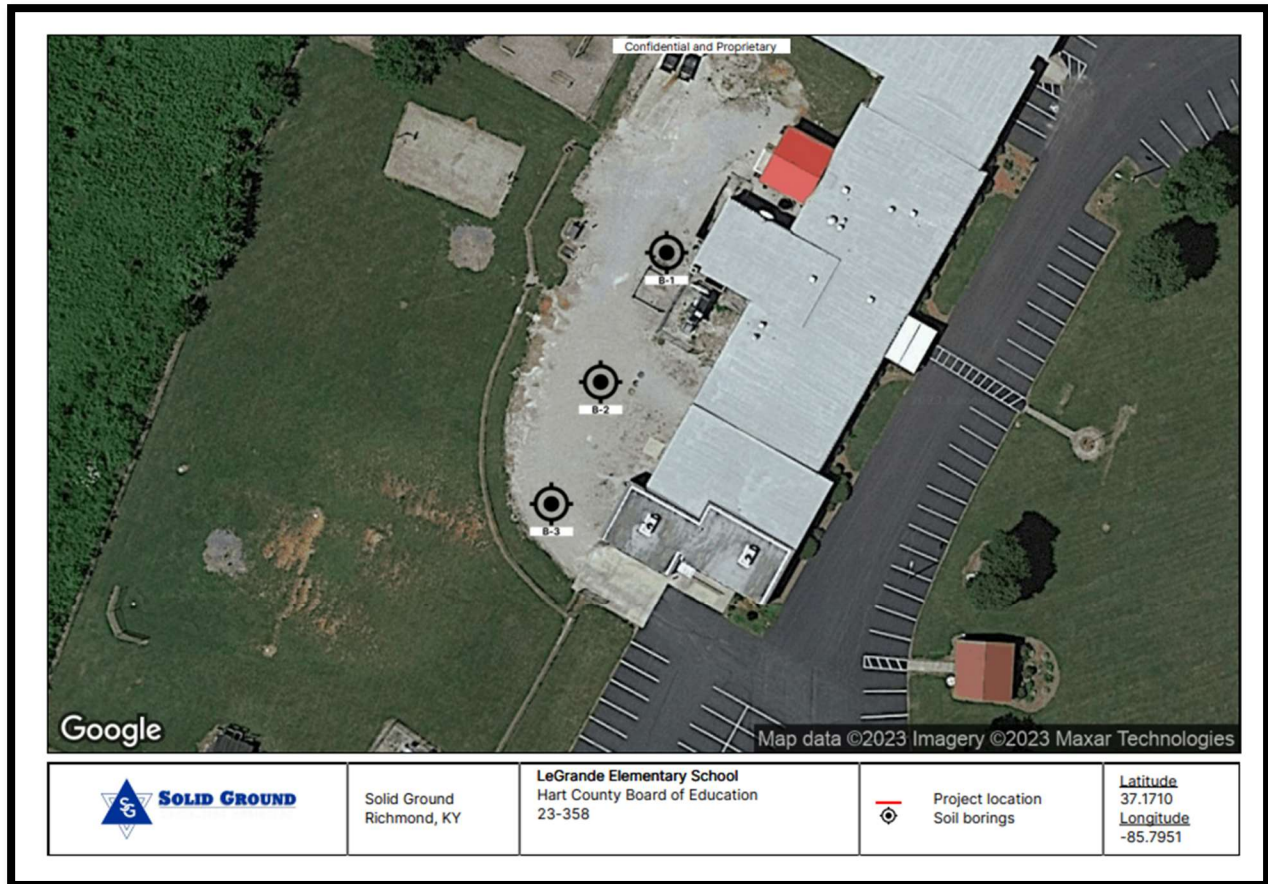
Figure 7: Approximate Boring Locations
